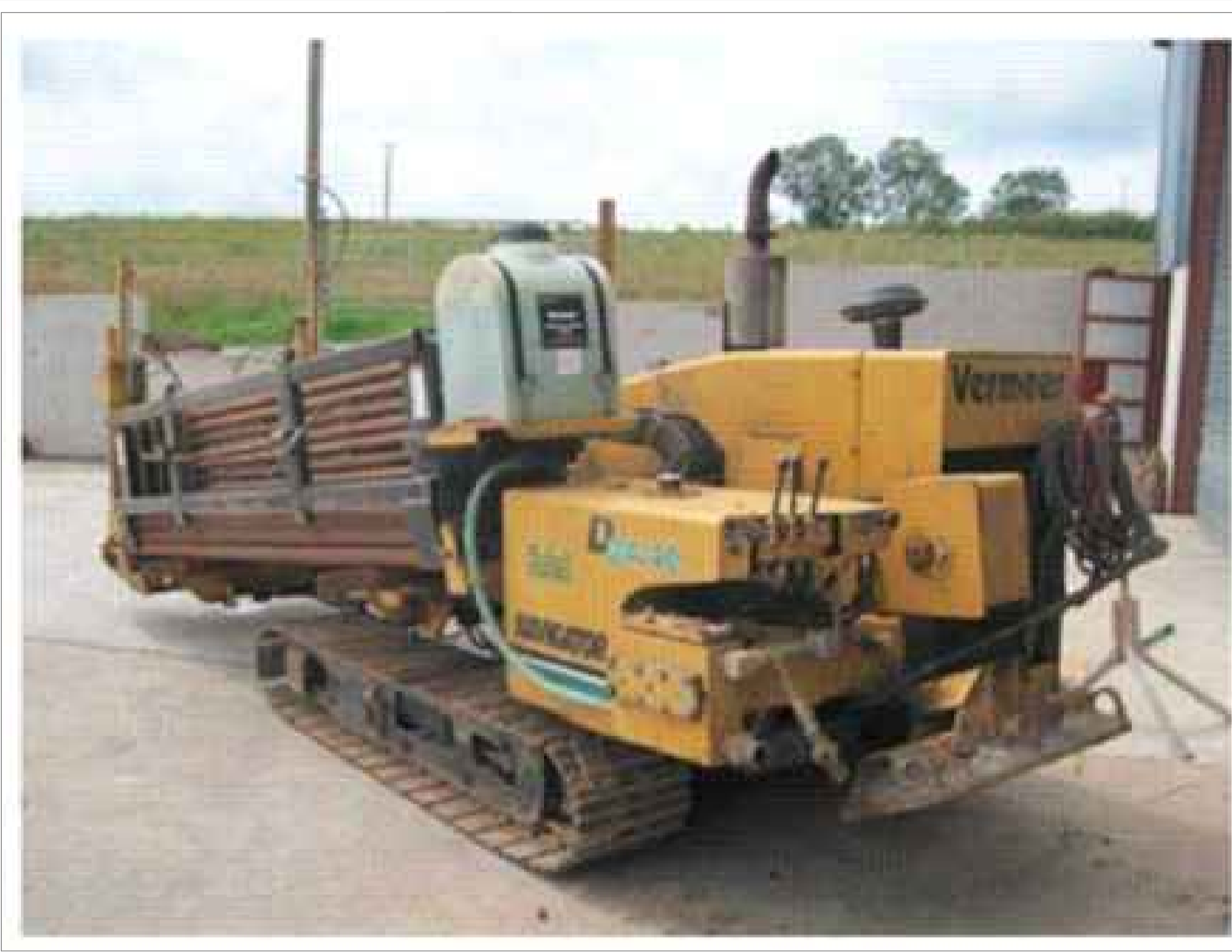
Image 2 | Typical Horizontal Directional Drilling Rig
